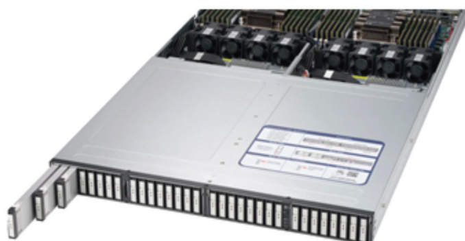
Figure 2: Supermicro® Server with 32 E1.L fitted in 1U chassis
